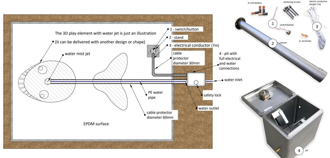
The delivery does not include the cable protector or the PE water pipe!
